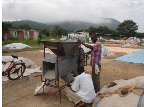
*Fig. 5. Simple Hand Operated Seed/Grain Cleaner From Ghana. These are usually manual operated as it can be difficult to gear down power ones sufficiently to prevent the grain from being blown away.*
