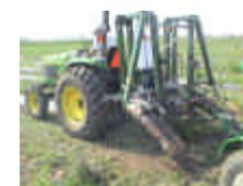
The Atarus Stinger with the steam nozzles positioned parallel to the strawberry bed.
