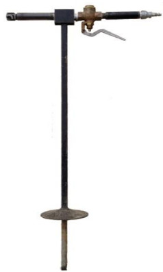
Figure 2. Soil injection needle used to deliver insecticide to the root zone of the plants. Photo by Melissa Franklin.
