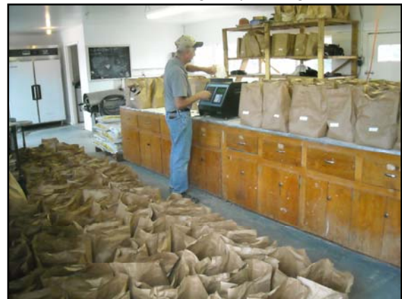
Calvin Pearson determining grain moisture and test weight on the Hayden wheat samples at the WCRC at Fruita. Photo by Fred Judson.
