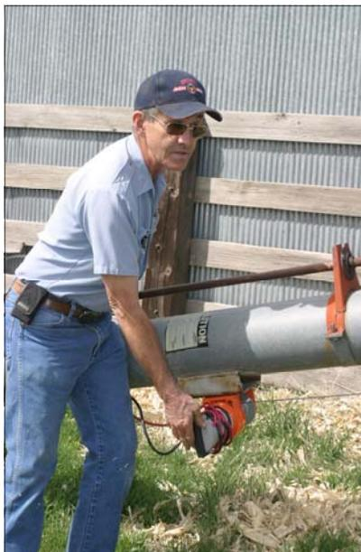
Mr. Frihauf using electric winch to raise and lower his auger.
