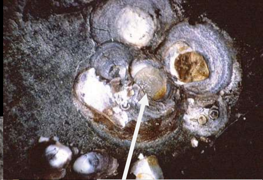
Cover removed to expose developing scale
