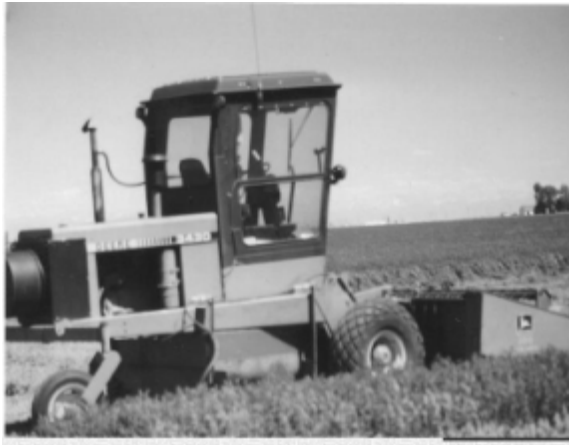
Fig.2 The John Deere 3430 crimper/swather with electronic weigh box added to weigh individual plots.
