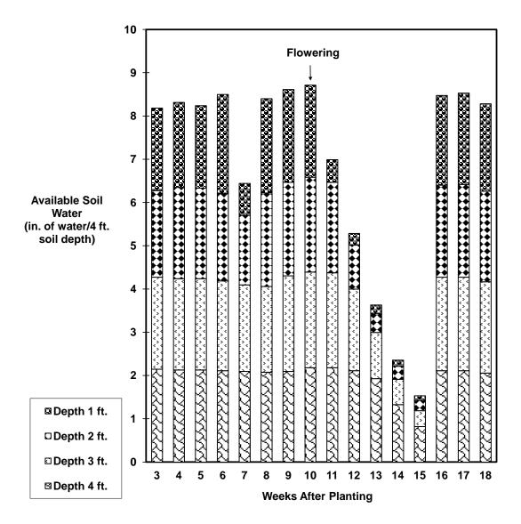
Fig. 1. Available soil water in dryland grain sorghum at Walsh. Gypsum block measurements taken to 4 ft. with 1 ft. increments. Total rainfall at Walsh from planting to first freeze was 15.59 in. Any increase in available soil water between weeks is from rain.
