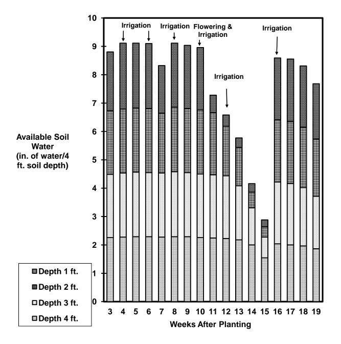
Fig. 2. Available soil water in drip irrigated grain sorghum at Walsh. Gypsum block measurements taken to 4 ft. with 1 ft. increments. Total rainfall at Walsh from planting to first freeze was 15.59 in. Any increase in available soil water between weeks not attributed to irrigation is from rain
