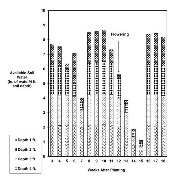
Fig. 3. Available soil water in dryland forage sorghum at Walsh. Gypsum block measurements taken to 4 ft. with 1 ft. increments. Total rainfall at Walsh from planting to harvest was 15.59 in. Any increase in available soil water between weeks is from rain.
