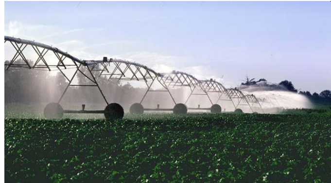
Fig. 15. Self-Propelled Center Pivot Irrigation System Commonly Use in the USA to Irrigate 48 ha of a 65 ha square. The Field is Cotton
