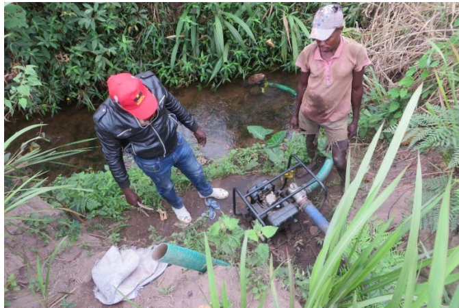
Fig. 9. Small Diesel Pump Used to Lift Water from Small Stream to Irrigate Adjacent Land Planted to Vegetables.
