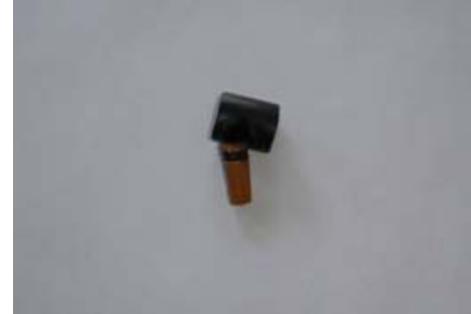
Fig. 32. Freak Accident Of Cigarette Butt Melted Hole In Drip Line Highlighting Potential for Careless Laborers Damaging Line.
