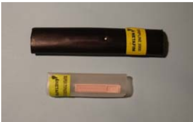
Fig. 20. Example of Commercial Embedded Emitters Including Transparent Sample Showing Torturous Track the Water Must Cover Before Exiting the Emitter. All This to Reduce Pressure and Allow Dripping Instead of Spraying.
