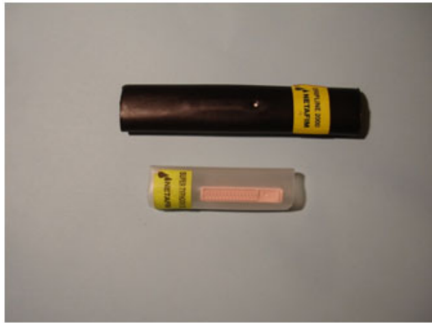
Fig. 2. Behind the clearly visible hole is a tortuous track pressure compensator in a typical drip emitter.
