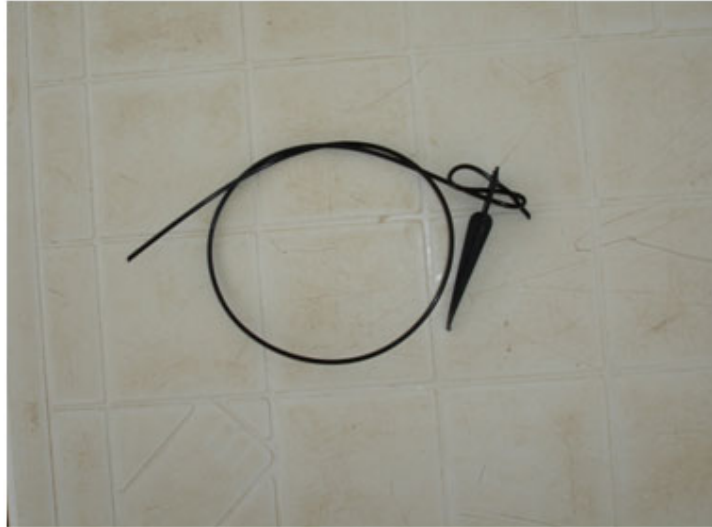
Fig. 3. Alternative emitter manufactured in Zambia with the pressure controlled by simply tightening the loop.
