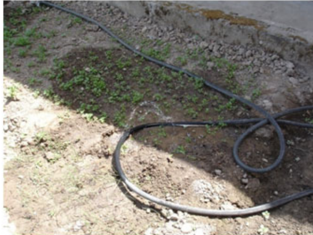
Fig. 1. Water spouting from a simple hole in a hose with no means for pressure compensation.
