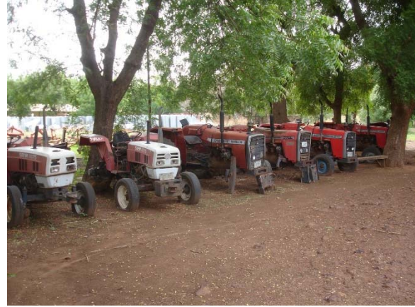
Fig.15. Typical Line of Surveyed Out of Operations Tractors With Less Than Half The Designed Operating Hours Outside any ADP In Nigeria.
