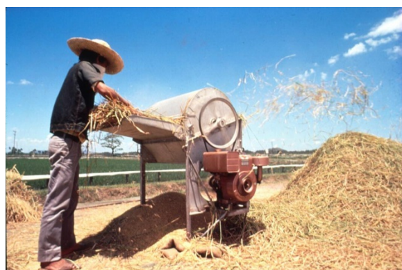
Fig. 2. IRRI axial flow thresher in use in the Philippines. IRRI file photo.
