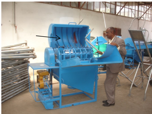
Fig. 1. IRRI style axial flow thresher being fabricated at Selam Childrens Village. Note baffles in top to guide cut grains.
