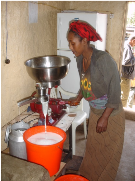
Fig. 20. Manually Operated Centrifuge for Separating Butter Fat from Milk
