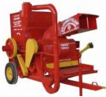
Fig. 6. Turkish thresher now widely used in Egypt for multiple crops.
