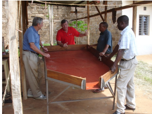
Fig. 13. A Cleaning Screen Designed by FtF Volunteer(at back) for Sunflowers prior to Extruding Oil in Kenya.
