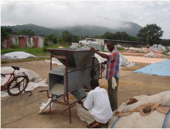
Fig. 9. Manual mechanical winnower used in Ghana for rice.
