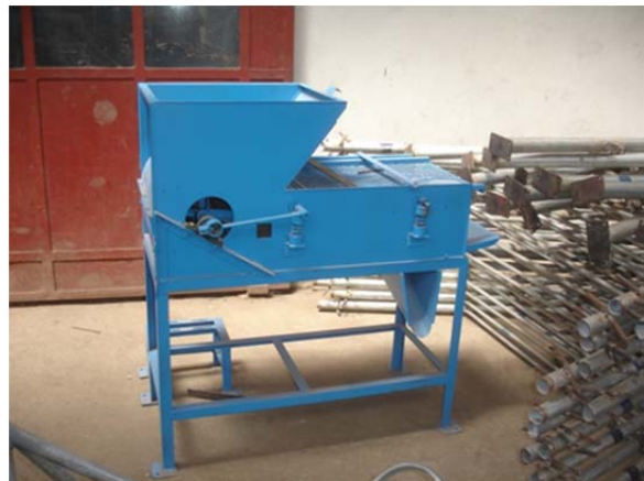
Fig. 8. Grain cleaner being fabricated by Selam Children's village. Requires a small petro engine.
