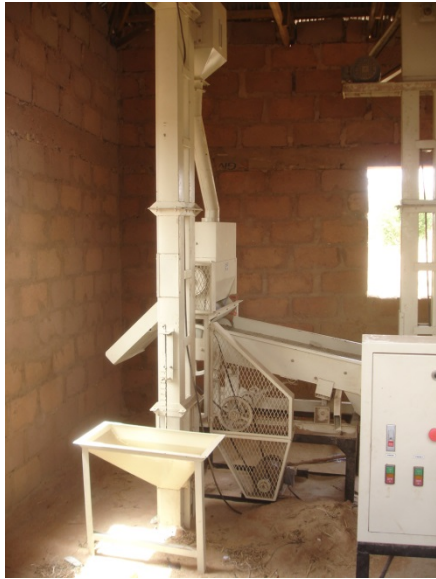
Fig. 12. Destoner In Front of Rice Mill to Remove Stones and Mud Clods Prior to Milling.
