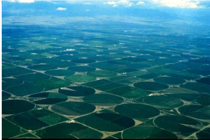
Fig. 18. Aerial View of Center Pivot Irrigation in San Luis Valley of Colorado. Each circle represents 50 irrigated ha. in a 72 ha square.
