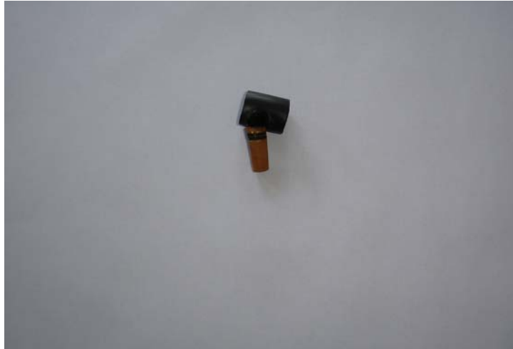
Fig. 26. Cigarette accidentally discarded against my home drip line melted a 6 mm hole in the line.
