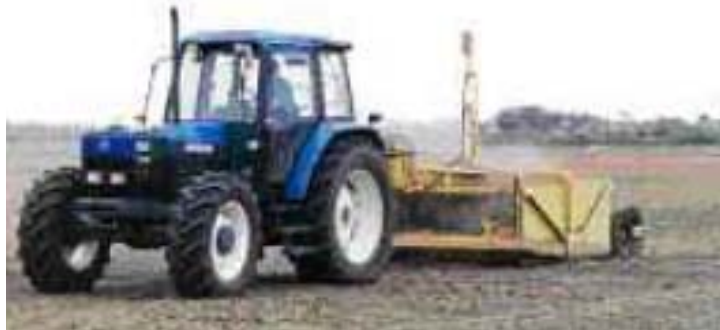
Fig. 16. Laser guided scraper with laser target mounted on scraper automatically controlled by the tractors hydraulic system.
