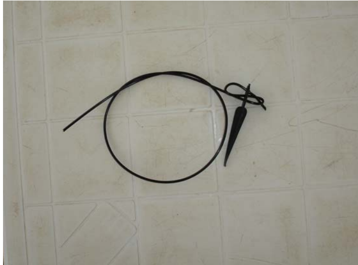
Fig. 22. Alternative emitter manufactured in Zambia with the pressure controlled by simply tightening the loop.
