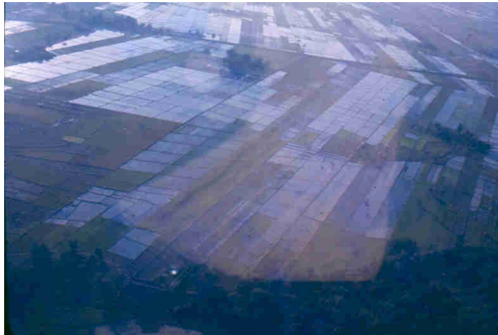
Fig. 2. Aerial View of Central Luzon Philippines where farms can be 1 km x 10 m to allow individual access to both the irrigation canal and drain.
