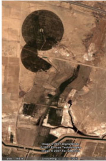
Fig. 7. Two center pivots pirating water from the secondary canal.
