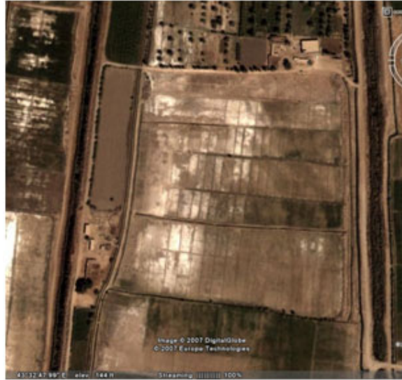
Fig. 10. Saline affected soils with characteristic salt visible on the surface.
