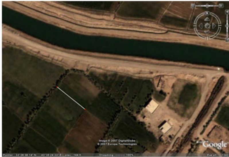
Fig. 9. Field layout showing field of less than one hectare further divided into small irrigation basins. The line represents 57 m.
