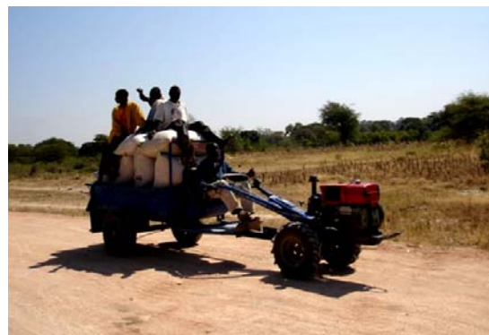
Fig. 16. Power tiller in Madibira, Tanzania overloaded in bringing rice plus laborers home for fields.
