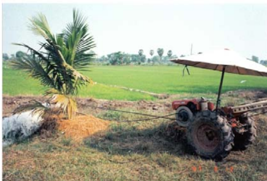
Fig. 15. Power tiller in Thailand being used for low lift pumping into rice fields.
