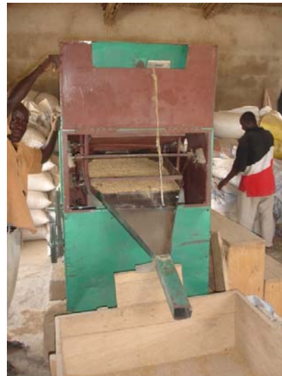
Fig. 13. Destoner placed in front of rice mill in Fig. 12 to remove stones and mud clods from the paddy prior to milling.
