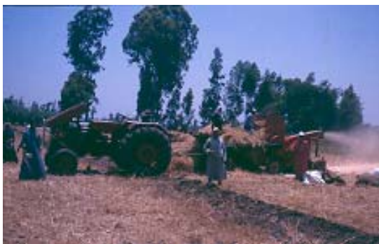
Fig. 7. Turkish Thresher Commonly used for both rice and wheat in Egypt but requiring a full 60hp Tractor for power.
