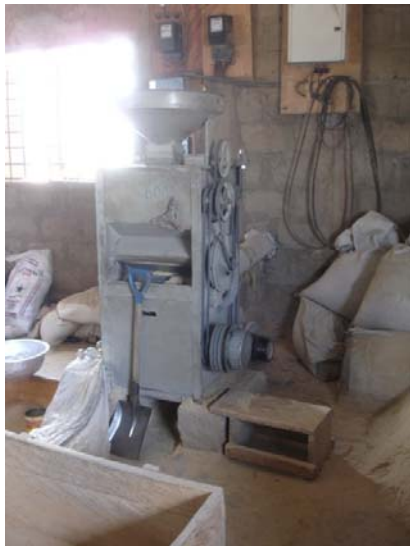
Fig. 12. Simple single pass, two stage rice mill used extensively in the scheme.
