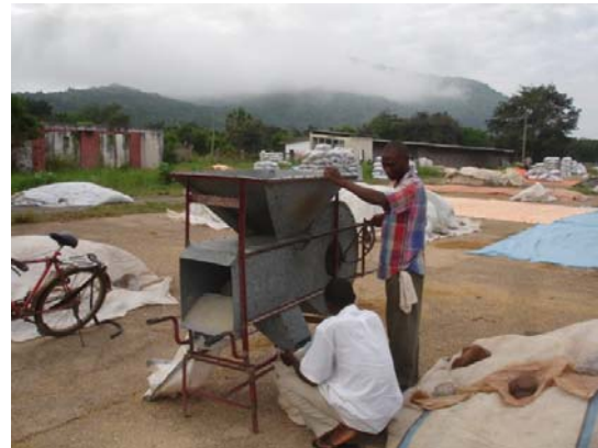
Fig. 11. A simple manually operated winnowing machine being used in the scheme. Such machines should make winnowing faster and more effective and should be encouraged.
