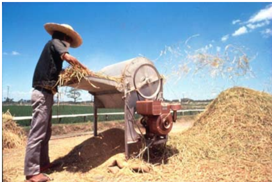
Fig. 6. Small axle-flow thresher developed by IRRI for threshing rice. Photo credit: IRRI
