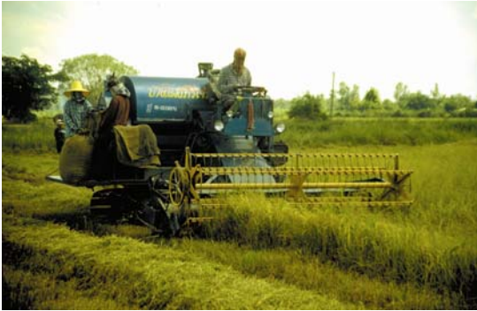
Fig. 8. Small combine designed specifically for smallholder rice fields. It is currently widely used throughout fully irrigated areas in Asia and allows much cleaner recovery of paddy and faster crop conversions.
