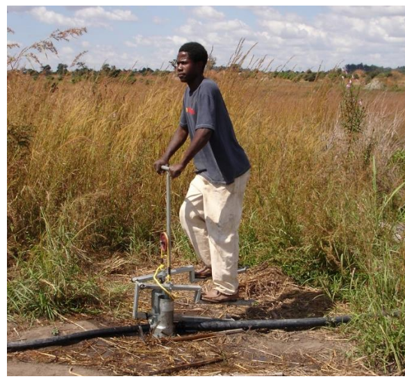
Fig. 4. Treadle pump distributed by NGOs for local small scale irrigation. But requiring people with limited dietary calories to work hard, perhaps well in excess of available calories.
