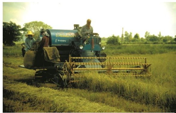
Fig. 7. Small combine commonly used in irrigated rice in Thailand that allow for increased rice cropping intensity.
