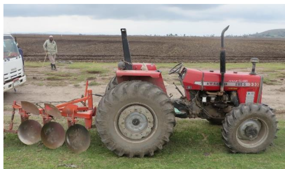
Fig. 8. Typical 60 to 80 hp tractors used by private service providers for contract land preparation slowly becoming available in many countries in Africa.
