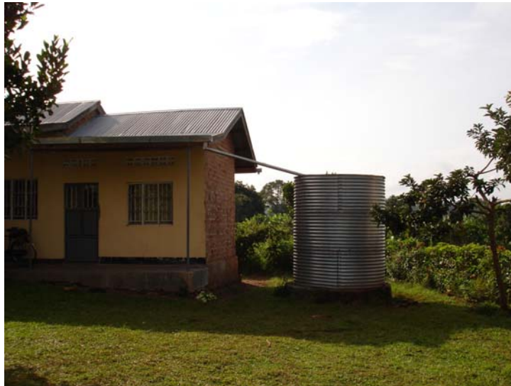
Fig. 9. Water harvesting from the roof at the RUCID center.
