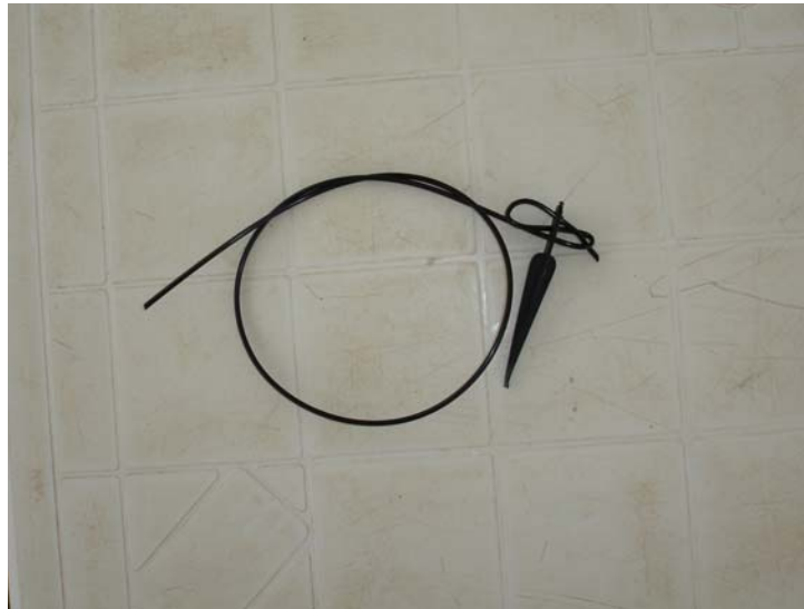
Fig. 14. Drip emitter manufactured and available in Zambia
