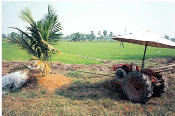
Fig. 2. Power Tiller Use for Low Lift Pumping From Canal In Thailand
