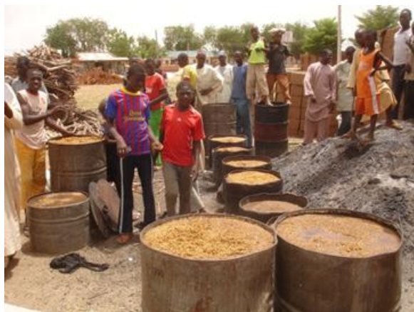
Fig 27. Paddy Soaking in 42 gal (160 lit) Barrels Used for Parboiling
