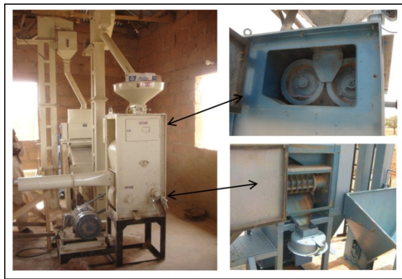
Fig. 34. Sakata Two Phase Mill Showing Roller Bars for Dehulling & Rasp Bar Drum for Polishing
