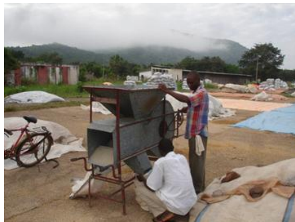
Fig. 24. Simple Manually Operated Winnowing Machine That Can Improve the Quality of Paddy.
