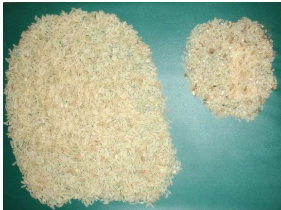
Fig. 32. Physical Separation of Head Rice From Broken and Other Material for Rice Milled In Single Phase Mill.
