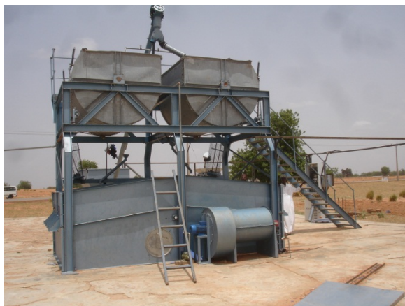
Fig. 59. Steam Injected Parboiling Vats above Forced Air Dryer at Abandoned Mill.
