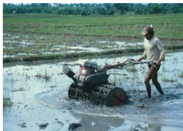
Fig. 1. Asian Rice Farmer Using Small Rice Based Power Tiller Ideal for Working in Paddy.
