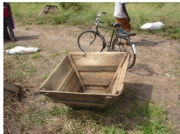
Fig. 19. Whacking box Used to Thresh Paddy in Ghana.
