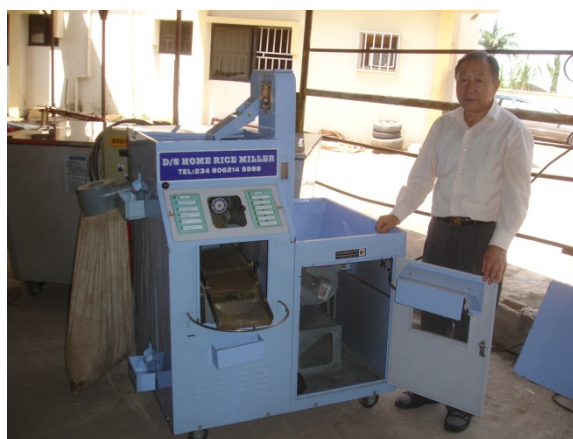
Fig. 60 Korean Manufactured 300 kg/hr. Destoning Rice Mill.
