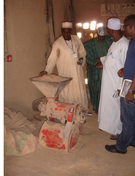
Fig. 31. Single Phase Mill Used for Rice But With Only 50% Recovery and Excessive Broken
