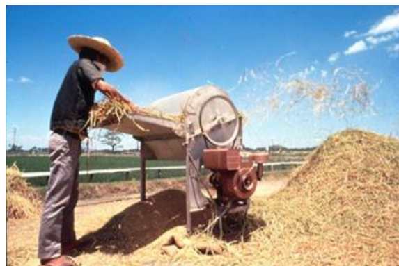
Fig. 21. IRRI Designed Axial Flow Thresher That Can Expedite Threshing and Increase the Recovery.
