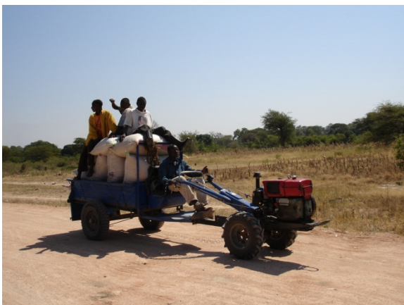
Fig. 52. Power Tiller With Trailer Used for Hauling Rice from Field To Home In Madibira, Tanzania.
