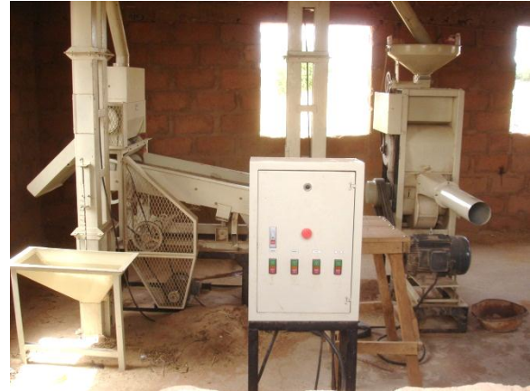
Fig. 33. Recently Obtained Sakata Two Phase Mill (Right) with De-Stoner (Left) in Kalambaina, A Rice Processing Community Near Sokoto
