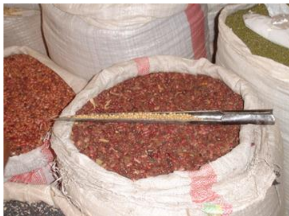
Fig. 42. Grain Spike (Thief) Used to Check Quality in Bags Of Any Grain
