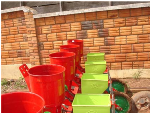
Fig. 13. Poorly Designed and Constructed Chinese Seeder that Needed Complete Overhaul to be Field Worthy.
