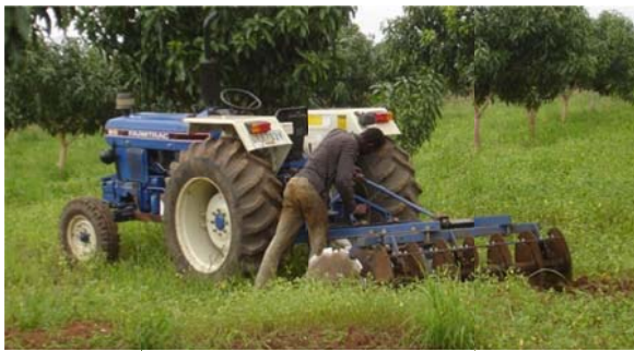
Fig. 16. Close up of Harrow to illustrate how the two rows of disc counteract to minimize soil movement.
