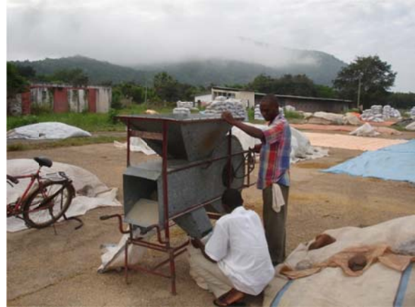
Fig. 20. Simple Manually Operated Winnowing Machine that Could Help Reduce Foreign Material in Soybean and Increase Value by 10% or More.
