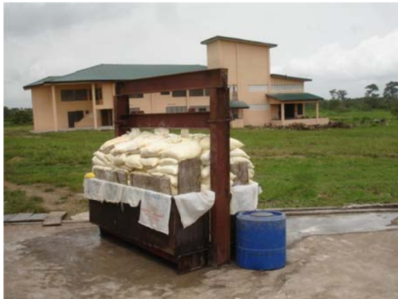
Fig. 14. Large Cassava Press Fabricated from Scratch by Caltech Mechanics.
