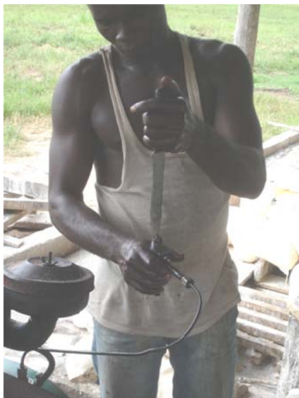
Fig. 15. Improvising Using a Large Knife to Adjust a High Pressure Diesel Fuel Injector.
