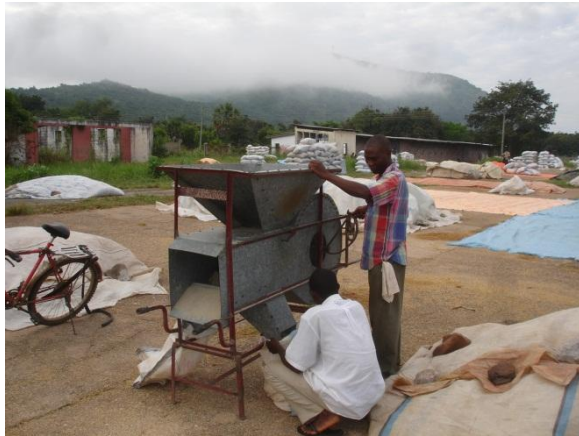
Fig. 5. Simple hand operated seed/grain cleaner from Ghana. These are usually manual operated; it can be difficult to gear down powered ones sufficiently to prevent the grain from being blown away.
